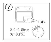
7.Observe the air pressure gauge, if the air pressure is lower than 180kPa, perform the inflation operation, then drive for 3-5km and check the tire pressure. If the tire pressure still drops significantly, it means that the tire is seriously damaged, which is beyond the scope of repair by the product. Which in this case, you will need to go to a car repair shop for instant assistance. If not, which means the tire is perfectly gets fixed.
