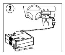
2.Insert the cigarette lighter into the car power socket, then start the car engine.
