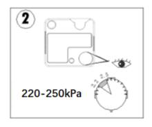
2.Observe the air pressure measure the tire pressure.
