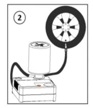
3. Insert the cigarette lighter into the car power socket, then start the car engine.
