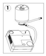
1.Make sure the on-off button is off. Loosen the sealant hose on the tire sealant bottle and the inflation hose on the inflator, connect the inflation hose to the air inlet of the sealant body, and then align the tire sealant bottle interface with inflator and push it in horizontally.
