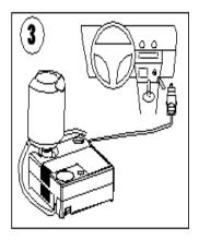
3.Insert the cigarette lighter into the car power socket, then start the car engine.
