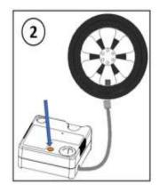
2.Press the pressure relief valve button (yellow) and observe the air pressure gauge until the tire pressure reduce to the desired value.
