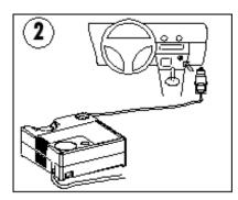
2.Insert the cigarette lighter into the car power socket, then start the car engine.
